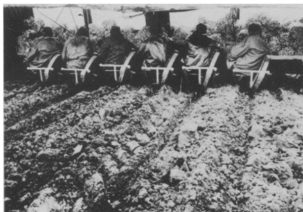
Figure 3. A planting machine with 6 rows is used for planting the willows. The rows are 70 cm apart, distances in the row are 50 cm. The planting stock consists of unrooted cuttings with a length of 23 cm. (Photo: Rijksdienst voor de IJsselmeerpolders, Lelystad).
